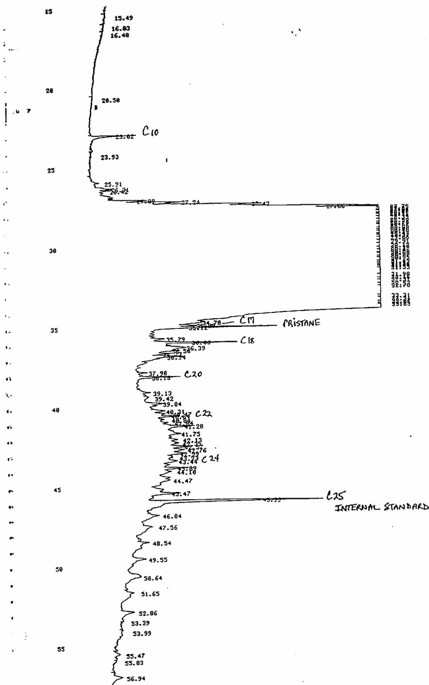
Figure 18. Non-saponifiables of mussel sample No. 2 in hexane analysed by liquid injection on a gas chromatograph.
