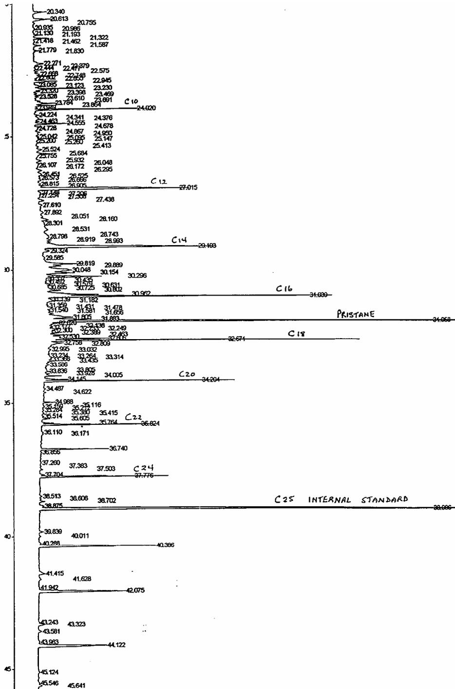
Figure 9. Non-saponifiables of rock crab flesh in hexane analysed by liquid injection on a gas chromatograph.
