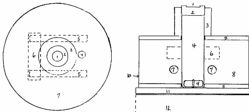
Top view: 1,PTFE/silicone septum; 2, phenolic screw cap; 3, Teflon collar; 4, thermometer well; 5, 80 watt electric heater; 6, 5 amp thermostat.
