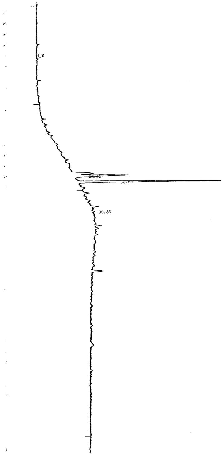
Figure 5. Headspace of vortexed distilled water analysed by gas chromatography.
