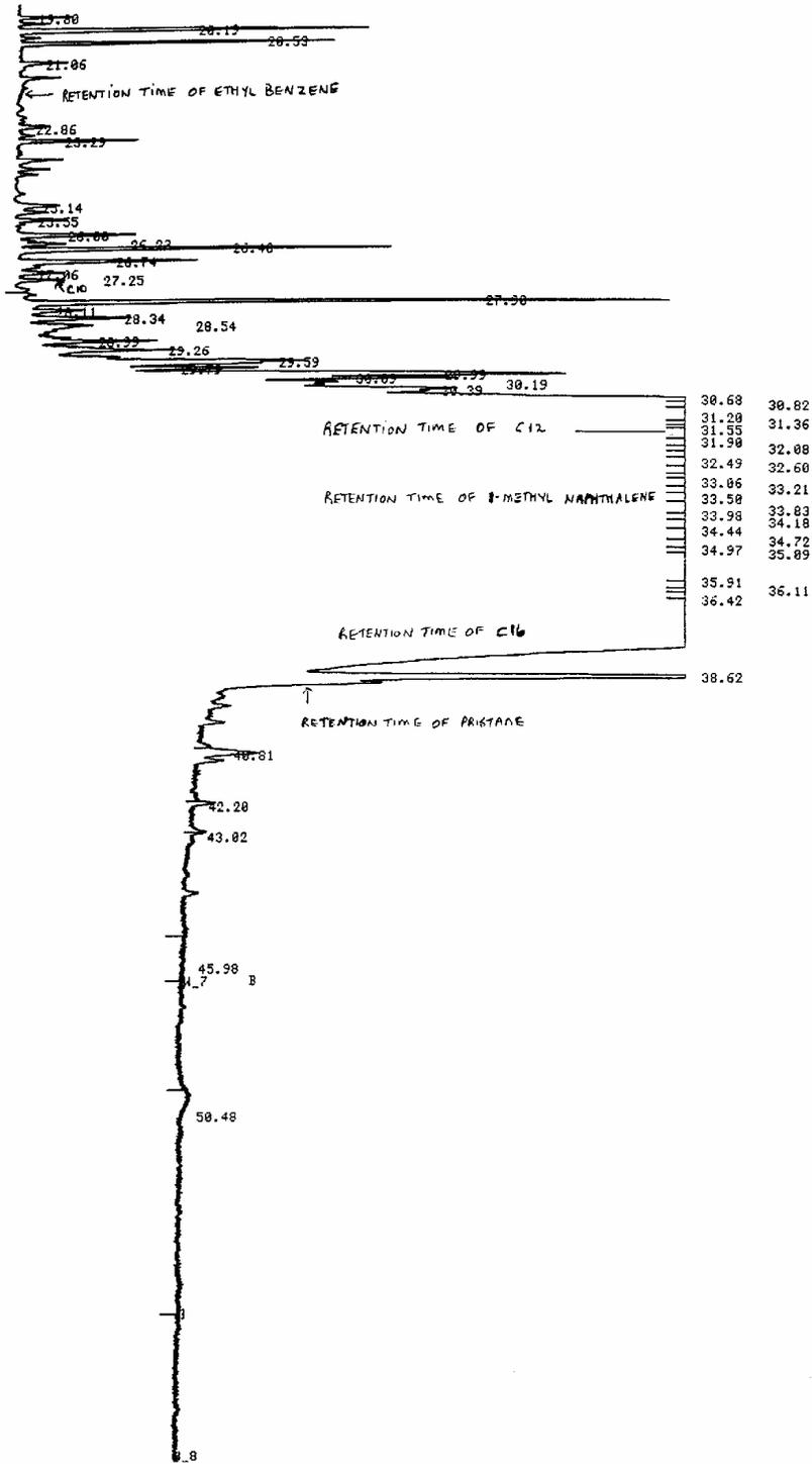
Figure 17. Headspace of mussel sample No. 2 in vortexed distilled water analysed by gas chromatography.
