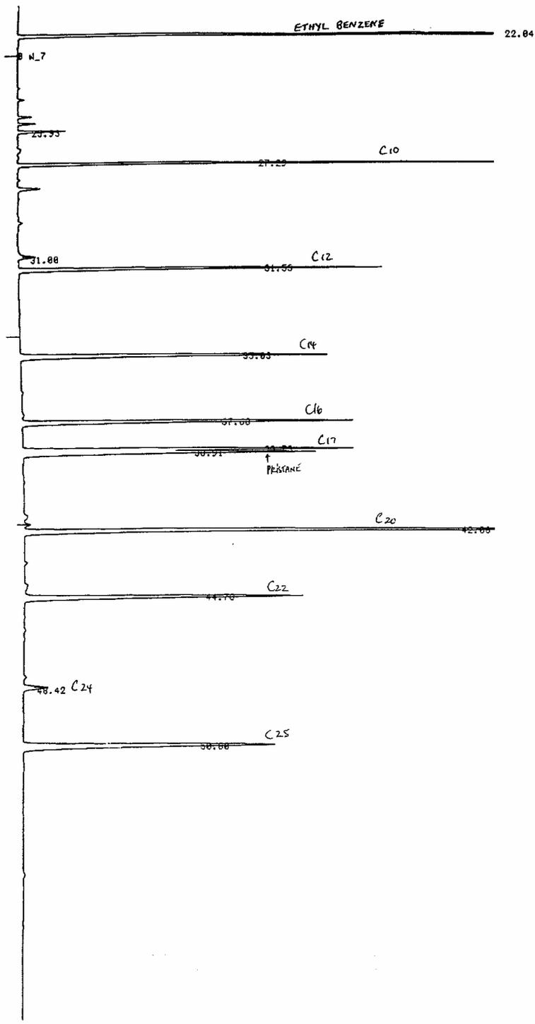
Figure 6. Liquid injection of standard mixture in dichloromethane analysed by gas chromatography to verify retention times of component hydrocarbons.
