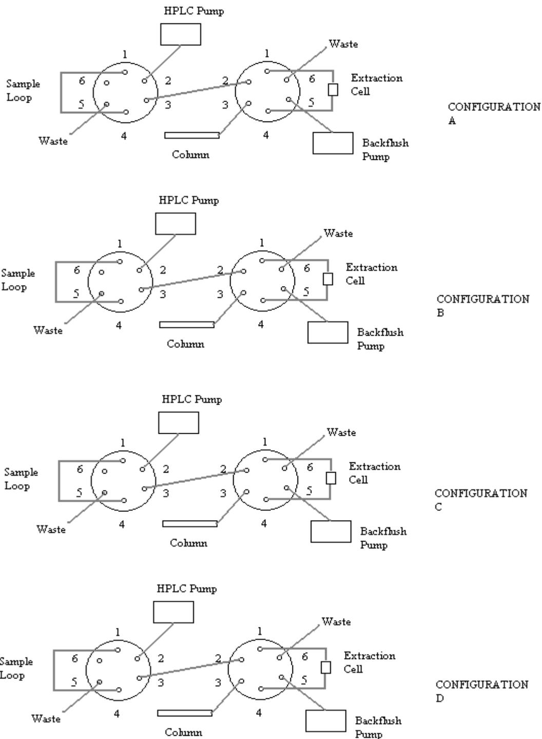
**Figure 2.3.** Schematic description of the injection system for online microfiltration analysis.
