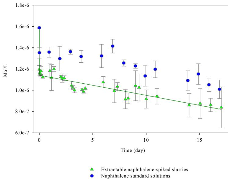
**Figure 3.9.** Dissolved and extractable naphthalene kinetic curves of HISS-1 slurries. Initial naphthalene concentration  $1.6 \times 10^{-6}$  M at  $25.0^{\circ}\text{C}$ . **(A)** Dissolved naphthalene, **(B)** Extractable naphthalene. Curve fitted using least square regression (naphthalene standard) and exponential decay (naphthalene-spiked slurries).
