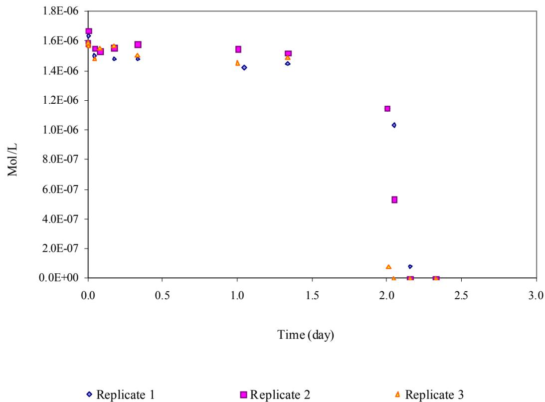
**Figure 3.3.** Extractable naphthalene concentration curves from triplicates naphthalene-spiked PACS-2 slurries. Initial naphthalene concentration:  $1.6 \times 10^{-6}$  M at 25.0°C. Free-hand curve fitted.
