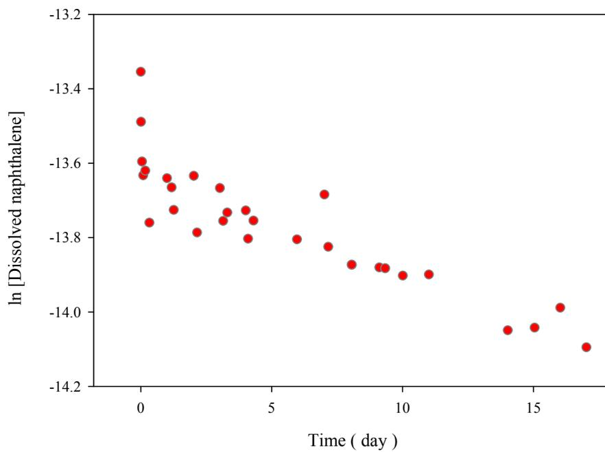
**Figure 3.11.** Natural logarithm of the dissolved naphthalene concentration vs. time for HISS-1 slurries. Initial naphthalene concentration  $1.6 \times 10^{-6}$  M at  $25.0^{\circ}\text{C}$ .
