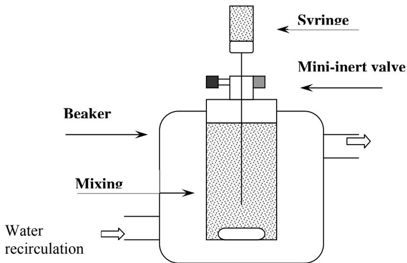
**Figure 2.1.** Schematic representation of mixing vessel
