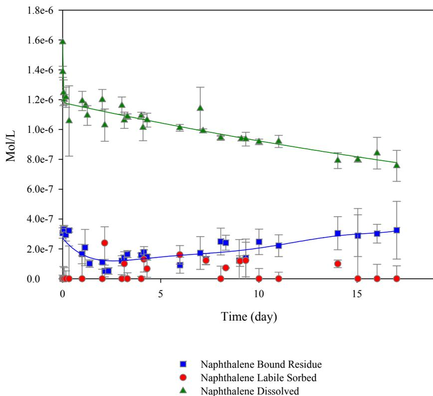
**Figure 3.10.** Dissolved, labile sorbed and bound residue naphthalene kinetic curves for HISS-1 slurries. Initial naphthalene concentration  $1.6 \times 10^{-6}$  M at  $25.0^{\circ}\text{C}$ . Dissolved naphthalene curve was fitted using exponential decay, labile sorbed naphthalene was free hand curve fitted, and bound residue naphthalene curve was fitted using least square regression.
