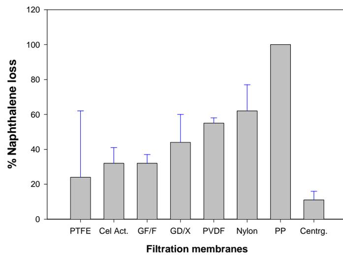
**Figure 2.6.** Naphthalene loss by sorption onto filtration membranes.
