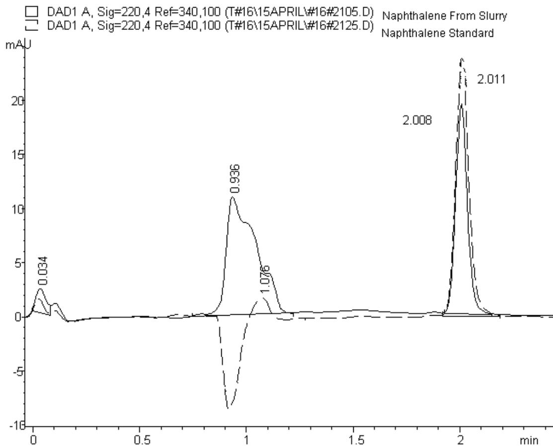
**Figure 3.13.** HPLC peaks of naphthalene and unknown peak. Aliquot offline centrifuged from  $4.0 \times 10^{-6}$  M naphthalene-spiked PACS-2 slurry at contact time  $t = 6.2$  day. Retention times: naphthalene: 2.0 min, unknown peak: 0.94 min. Dashed line: naphthalene standard, full line: naphthalene from slurry.
