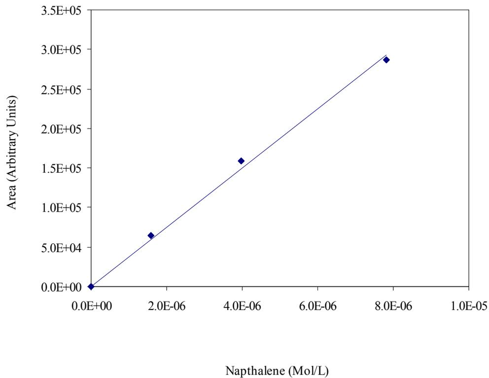
**Figure 2.5.** Calibration curve naphthalene standard solutions. Varian ProStar HPLC. Online microfiltration setup. Wavelength 220 nm. Best fit:  $\text{Area} = 3.74 \times 10^{10} [\text{Napthalene}]$ . Correlation coefficient  $r^2 = 0.996$ .
