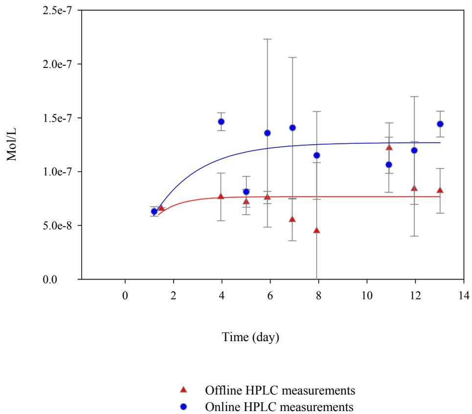
**Figure 3.12.** Naphthalene desorption kinetic curves of HISS-1 slurries. Initial naphthalene concentration  $1.6 \times 10^{-6}$  M at 25.0 °C. Curve fitted using exponential rise.
