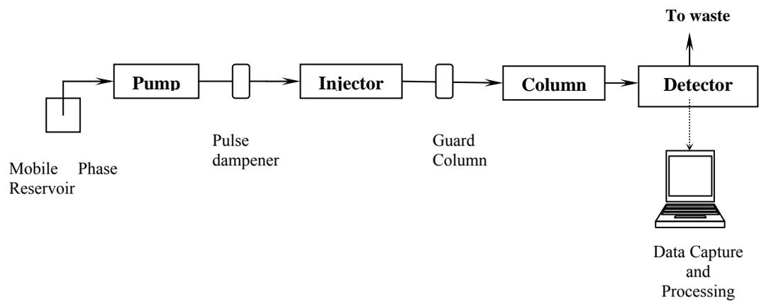
**Figure 2.2.** Block diagram of a conventional HPLC system
